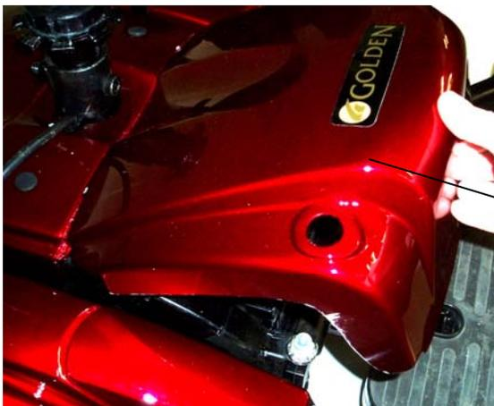
After removing the seat, locate the (2) "Battery Box Covers", on front and rear. Remove one of the covers by lifting up on the outer edge of the cover.
