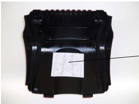
Note: On the inside of the battery box cover there is a battery connection diagram.
