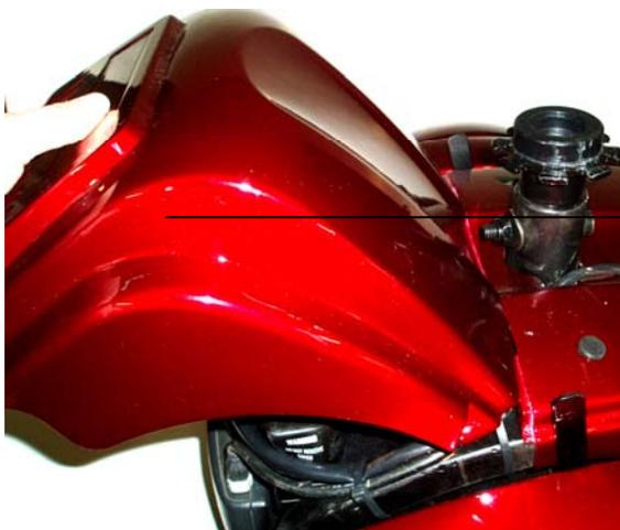
Remove the second "Battery Box Cover" by lifting up on the outer edge of the cover.
