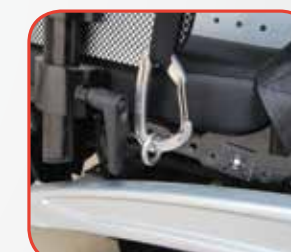
Snap the Karabiner onto the eye hole bracket
